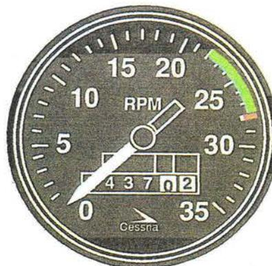
Figure 5-4. Tachometer
